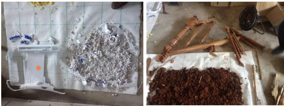
Figure 23: plastic (left) and wood (right), before and after fragmentation
