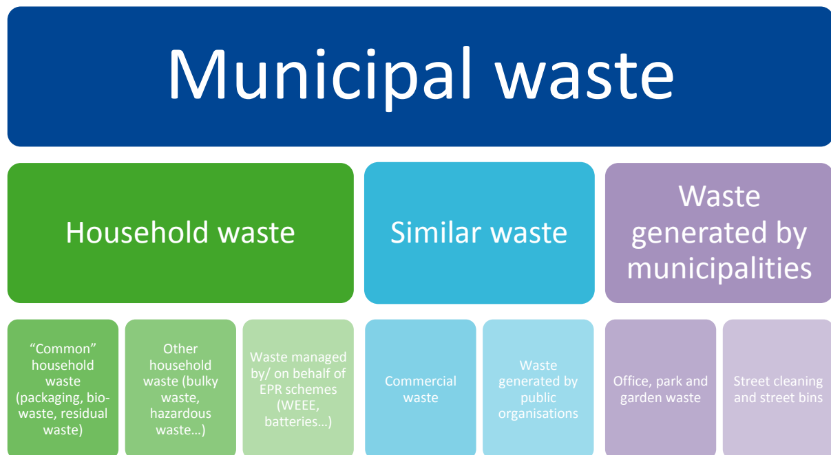
Figure 5: scope of municipal waste (EPR: Extended Producer Responsibility / WEEE: Waste Electronic and Electrical Equipment)
