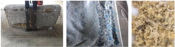
Figure 3. Fragmentation of mattresses: metal parts (springs), textile and foam
