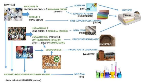
Figure 2 Streams and processes in URBANREC Project
