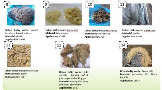
Figure 8. Materials from ECOFRAG forwarded to gasification (CHGP)
