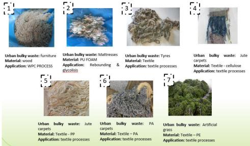
Figure 1. Fragmented streams approved for industrial applications
