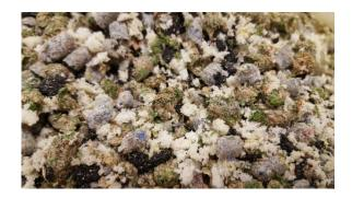
The gasification tests performed with this bulky waste mixture resulted in the syngas shown in the photo below.
