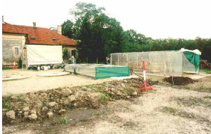
Figure: Emission measurement set up from ILEUT with big and small measuring unit. In the back the mobile measuring office
