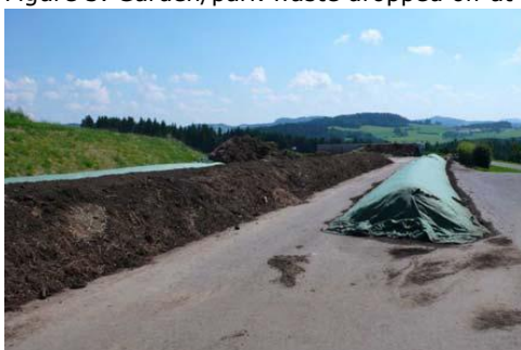
Figure 4. Typical on-farm composting site in Austria using open windrow technology with a cover/fleece
