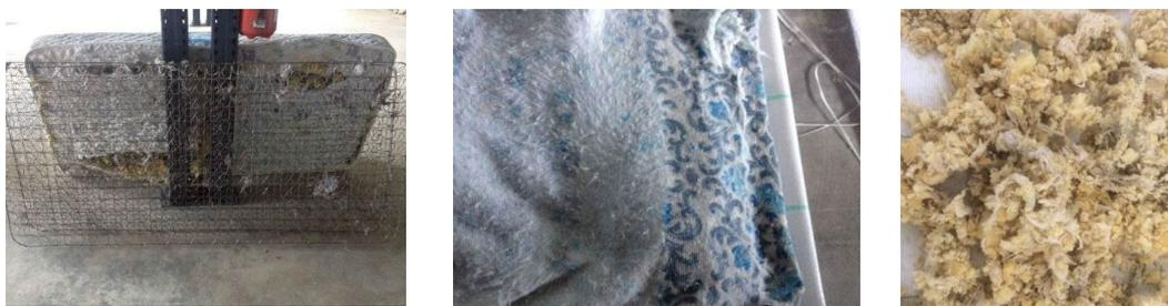
Figure 21: fractions separated from mattresses: metal, textiles, and foam
